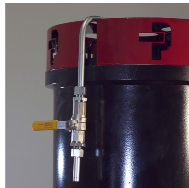
Optional safety cover prevents opening of a pressurized housing. Vent line comes with a ball valve.
